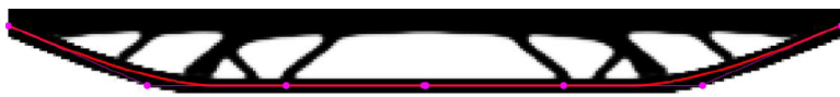
Figure 2: Optimized topology and tendon layout of a simply-supported beam, constant pre-stressing force T_{pre}^0 = 625
