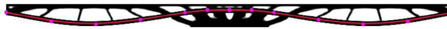
Figure 6: Optimized topology and tendon layout of a two-span beam, variable pre-stressing force T_{pre} = 842.941 and a curvature constraint \bar{\kappa} = 0.0035
